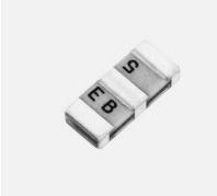
The CFECV Series are small, high performance and super thin (1.5mm) filters. Piezoelectric element is connected in the sandwich shape by heat resistant substrate. The filters exhibit flat G.D.T characteristic in pass band. The filters are recommended for digital communication application and are perfect in hand held cellular phones, pocket cordless phones, etc.
