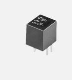
The CFU 455 line of ceramic filters are 4-element devices connected in ladder form while the CFWS 455 line of ceramic filters contain 6-elements. These compact, highly selective filters are recommended for use in applications ranging from two-way radio to auxiliary filters in high class transceivers. (Also available in 450kHz version.)
